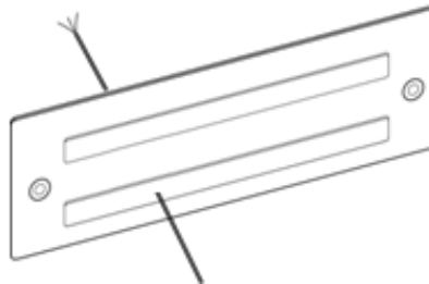
Figure 10 Schematic Diagram of a Feeding the Audio Output Cable through the Protective Terminal Cover
